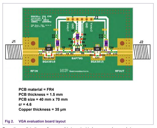
For optimum distortion performance it is important to have enough ground vias underneath and around the MMICs ground pins. This lowers the inductance to the ground plane. The evaluation board is made with two layer FR4 material.
