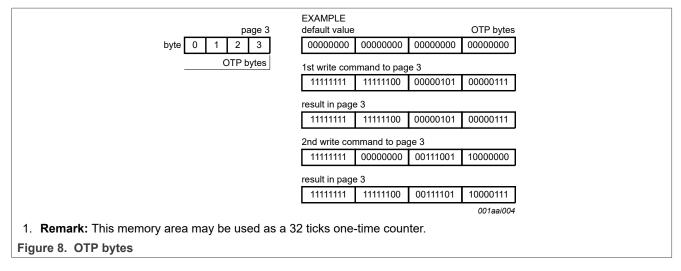
The bytes of the WRITE command and the current contents of the OTP bytes are bit-wise "OR-ed" and the result forms the new content of the OTP bytes. This process is irreversible. If a bit is set to "1", it cannot be changed back to "0" again.
