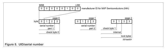
SN0 holds the Manufacturer ID for NXP (04h) according to ISO/IEC14443-3 and ISO/IEC 7816-6 AMD.1.
