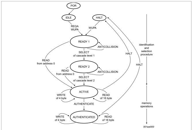
**Remark:** In each state the command interpreter returns to the Idle state if an unexpected command is received or any other error occurs. If the IC has already been in the Halt state before it returns to the Halt state in such a case. Those transitions are not explicitly shown in the state diagram.
