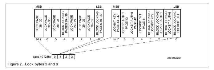
The default value of lock bytes 2 and 3 is 00 00h. The value of byte 3 on page 28h (see Figure 7) is always BDh when read.
