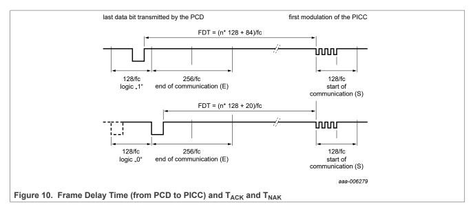
**Remark:** Due to the coding of commands, the measured timings usually excludes (a part of) the end of communication. Consider this factor when comparing the specified with the measured times.
