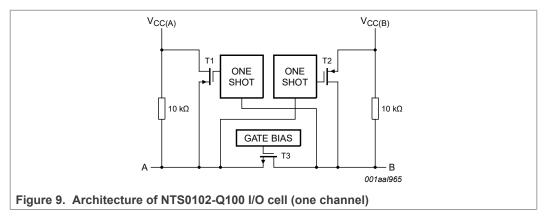
The NTS0102-Q100 is a "switch" type voltage translator, it employs two key circuits to enable voltage translation:
