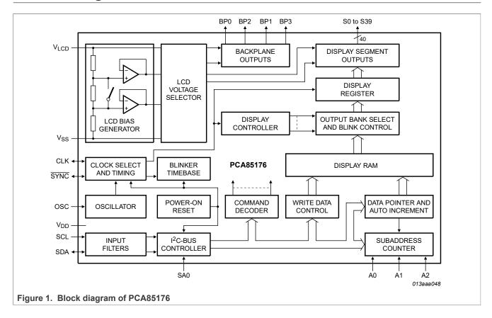
40 x 4 automotive LCD driver for low multiplex rates
