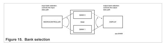
In the static drive mode, the bank-select command may request the contents of row 2 to be selected for display instead of the contents of row 0. In the 1:2 multiplex mode, the contents of rows 2 and 3 may be selected instead of rows 0 and 1. This gives the provision for preparing display information in an alternative bank and to be able to switch to it once it is assembled.
