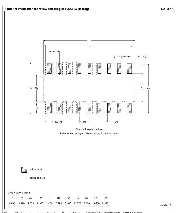
Figure 33. Footprint information for reflow soldering of SOT364-1 (TSSOP56) of PCA85176T
