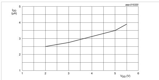
$T_{amb}$  = 30 °C; 1:4 multiplex drive mode;  $V_{LCD}$  = 6.5 V;  $f_{clk(ext)}$  = 1.536 kHz; all RAM written with logic 1; no display connected;  $I^2C$ -bus inactive.
