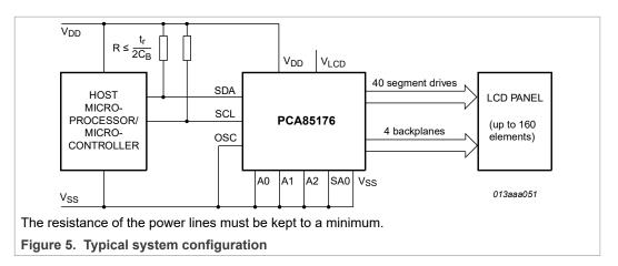
The host microcontroller maintains the 2-line  $I^2C$ -bus communication channel with the PCA85176. The internal oscillator is enabled by connecting pin OSC to pin  $V_{SS}$ . The appropriate biasing voltages for the multiplexed LCD waveforms are generated internally. The only other connections required to complete the system are the power supplies ( $V_{DD}$ ,  $V_{SS}$ , and  $V_{LCD}$ ) and the LCD panel chosen for the application.
