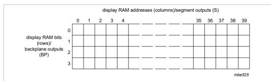
The display RAM bitmap shows the direct relationship between the display RAM column and the segment outputs; and between the bits in a RAM row and the backplane outputs.
