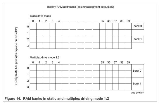
There are two banks; bank 0 and bank 1. <u>Figure 14</u> shows the location of these banks relative to the RAM map. Input and output banks can be set independently from one another with the Bank-select command (see <u>Table 9</u>). <u>Figure 15</u> shows the concept.
