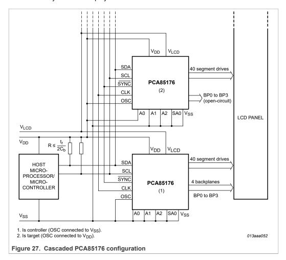
The SYNC line is provided to maintain the correct synchronization between all cascaded PCA85176. Synchronization is guaranteed after a power-on reset. The only time that SYNC is likely to be needed is if synchronization is accidentally lost (e.g. by noise in adverse electrical environments or by defining a multiplex drive mode when PCA85176 with different SA0 levels are cascaded).
