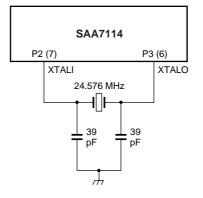
e. With fundamental quartz. Crystal load = 20 pF.
