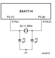
c. With fundamental quartz. Crystal load = 8 pF.
