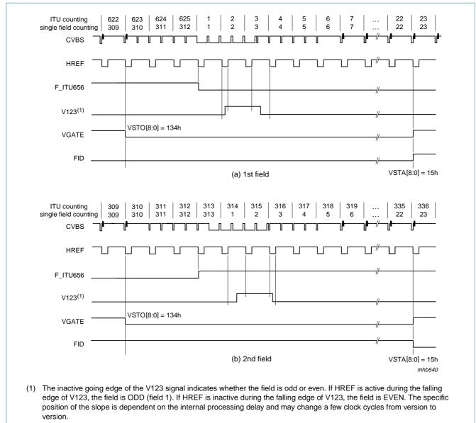
The control signals listed above are available on pins RTS0, RTS1, XRH and XRV according to <u>Table 8</u>. For further information see <u>Table 56</u>, <u>Table 57</u> and <u>Table 58</u>.
