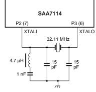
a. With 3rd harmonic quartz. Crystal load = 8 pF.
