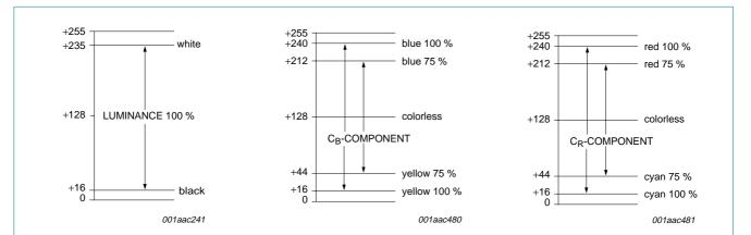
"*ITU Recommendation 601/656*" digital levels with default BCS (decoder) settings DCON[7:0] = 44h, DBRI[7:0] = 80h and DSAT[7:0] = 40h.
