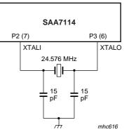
f. With fundamental quartz. Crystal load = 8 pF.
