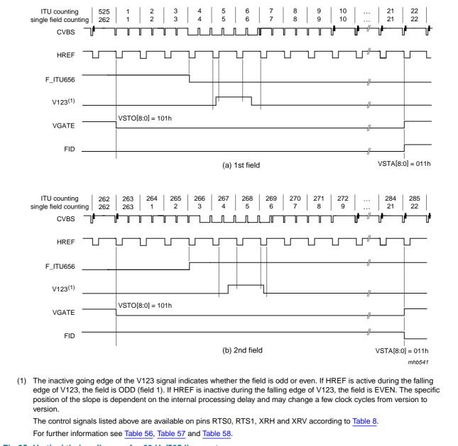
Fig 25. Vertical timing diagram for 60 Hz/525 line systems
