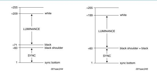
CVBS levels with default settings RAWG[7:0] = 64 and RAWO[7:0] = 128. Equation for modification of the raw data levels via bytes RAWG and RAWO:
