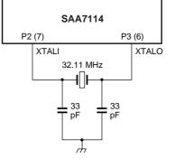
b. With fundamental quartz. Crystal load = 20 pF.
