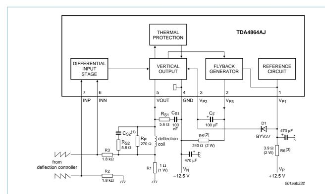
Attention: the heatsink of the IC must be isolated against ground of the application (it is connected to pin GND).
