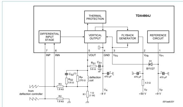
Attention: the heatsink of the IC must be isolated against ground of the application (it is connected to pin GND).
