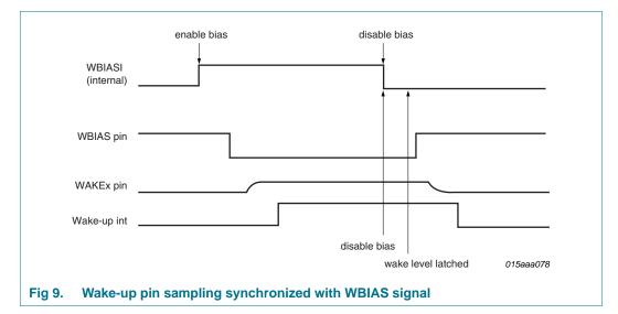
The sampling of the wake-up pins can be synchronized with the WBIAS signal by setting bits WSE1 and WSE2 in the Int\_Control register to 1 (if WSEx = 0, wake-up pins are sampled continuously). The sampling will be performed on the rising edge of WBIAS (see Figure 9). The sampling time, 16 ms or 64 ms, is selected via the Wake Bias Control bit (WBC) in the Mode\_Control register.
