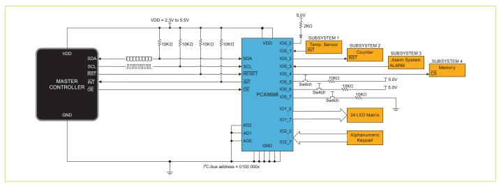
The  $1^2$ C-bus allows easy two-line communication between two devices using a serial data line (SDA) and a serial clock line (SCL) and, as a result, is a popular choice for computing, consumer electronics, communication, and industrial systems.
