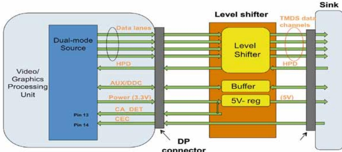
Most of the graphic sources in the market currently support Dual-Mode DisplayPort. This allows for using a simple level-shifter solution as the adapter. Level-Shifters convert the 3.3 V domain DisplayPort side source signal to a 5 V domain making it suitable for the sink side which supports DVI and HDMI. NXP offers a suite of DisplayPort to DVI and HDMI adapter solutions enabling adoption of DisplayPort in multiple applications.
