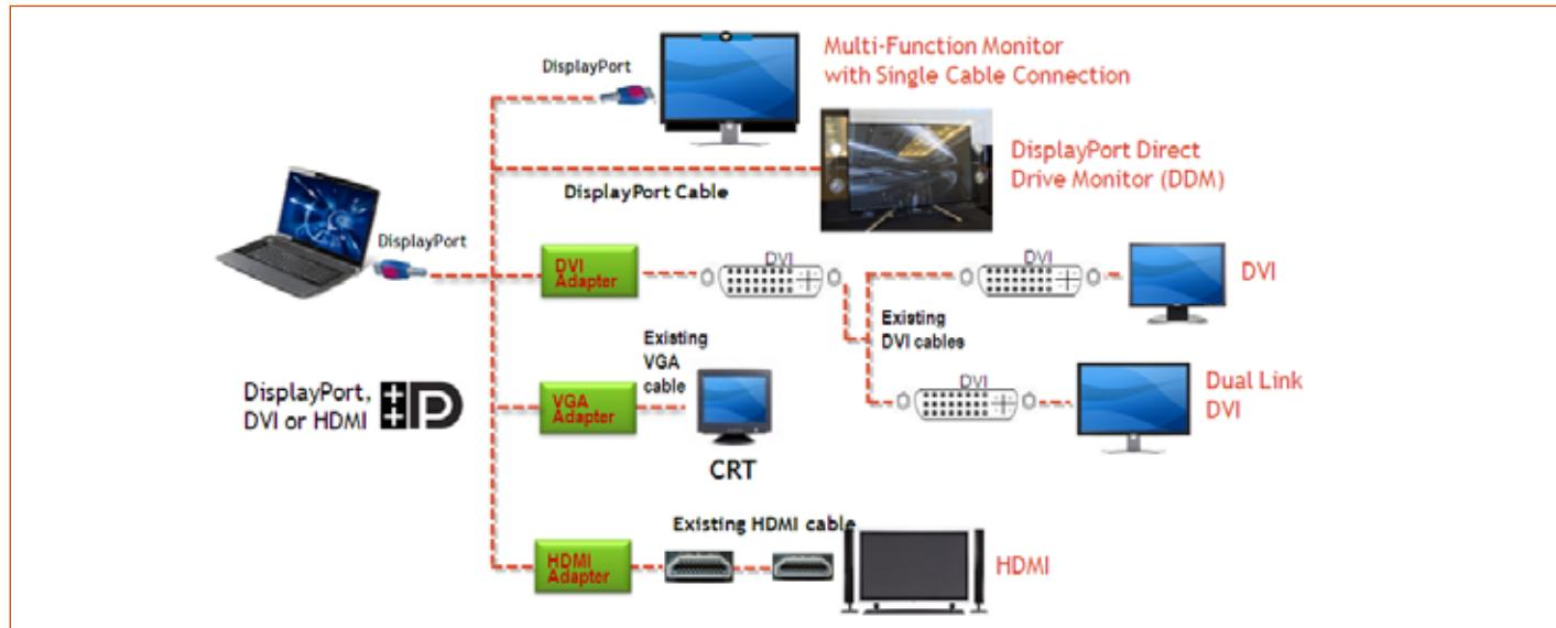
In order to support the trend to DisplayPort interconnectivity, NXP has developed several families of part types to address the growing demand for Level Shifters, Adapters, and Multiplexers used in Cable adapters and motherboards.
