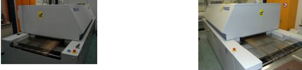
Figure 11 – Entry of the convection oven (left) and exit of the convection oven (right)
