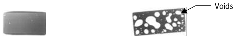
Figure 5 – The soldering surface before the soldering step (left) and after the soldering step (right) - No vacuum
