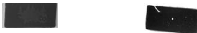
Figure 6 – The soldering surface before the soldering step (left) and after the soldering step (right) – vacuum
