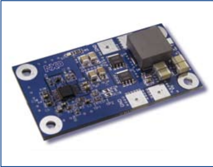
Implemented in a four-layer PC board, the 25-A POL converter measures 3.2 x 6.0 cm
