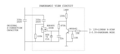
For a linear picture the digital control command must be a logic "1". The collector voltage of the MPSA42 will be low. The gate source voltage of the power MOS FET will be approximately -0.6V (FET switch open) and only one S-correction capacitor is active.
