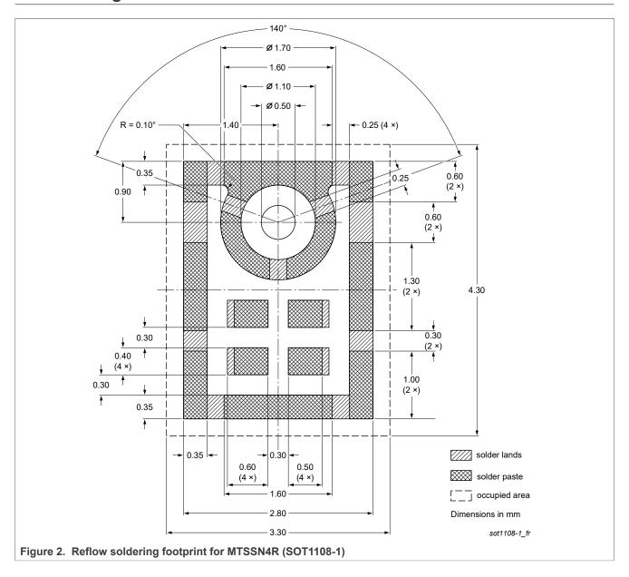
metal thin special-shape package; no leads; 4 terminals; resin based; body 4 mm x 3 mm x 1 mm
