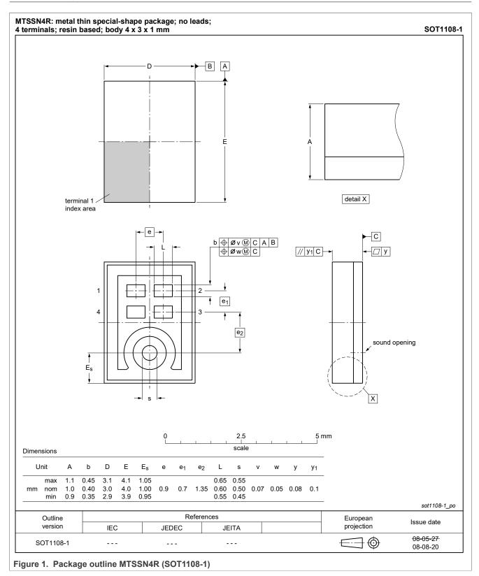
metal thin special-shape package; no leads; 4 terminals; resin based; body 4 mm x 3 mm x 1 mm
