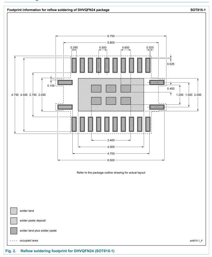
plastic, dual in-line compatible thermal enhanced very thin quad flat package; 24 terminals; 0.5 mm pitch; 3.5 mm x 5.5 mm x 0.85 mm body
