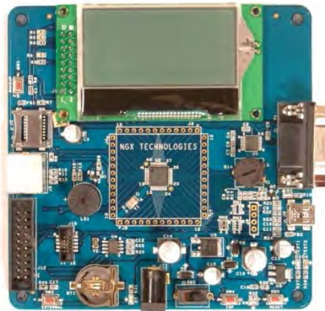
Fig 5. LPC1114 MCU based NGX board
