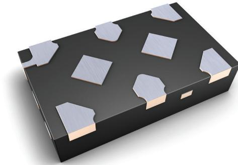
The GX-8 represents NXP's determination to offer compact, cost-effective packages that respond to the market's increasing demand for single- and dual-gate logic devices. The GX-8 has a pitch greater than 0.4 mm and thus maintains the DFM benefits associated with the 5- and 6-pin GX. But the additional pins offered by the GX-8 open up new opportunities for the inclusion of additional, more complex functions while saving board space and reducing assembly costs.
