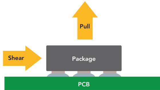
GX devices are leadless and thus share in this enhanced durability. However, the unique geometry of the 5-pin GX package creates an even higher contact-area-to-package-area ratio. This means that the GX family of packages may be not only the world's smallest but also the world's strongest logic package.
