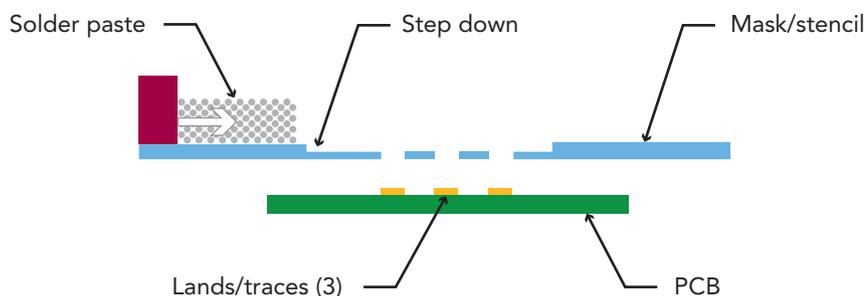
Second, the thickness of the solder stencil must be reduced. Reducing the stencil thickness leads to a corresponding reduction in the amount of solder deposited on the pad, and this smaller quantity of solder is less likely to form a bridge between adjacent pads. In order to ensure adequate mechanical strength and accommodate smaller or tighter pitch components, the assembly process for these components with very-fine-pitch will employ a so-called “step-down” stencil.
