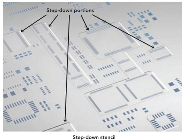
Such stencils are, of course, more complex to manufacture and therefore more expensive; they are also more fragile and may need to be replaced more frequently. In addition to the increased cost, the need for a step-down stencil imposes irksome restrictions on component placement—the smaller-pitch components must be located in PCB areas that correspond to the thinner sections of the stencil.
