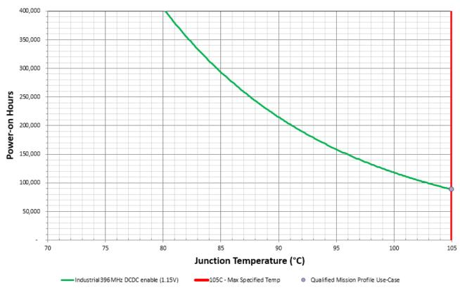
Figure 3. i.MXRT1020 Industrial lifetime estimates DCDC-enabled mode
