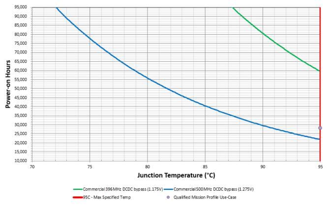
Figure 2. i.MXRT1020 commercial lifetime estimates, DCDC-bypass mode
