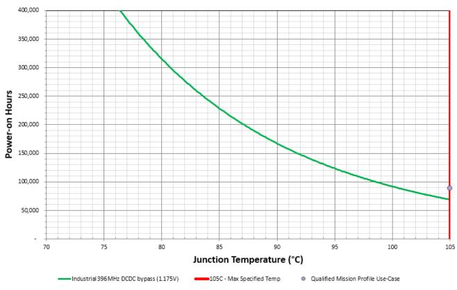
Figure 4. i.MXRT1020 Industrial lifetime estimates DCDC-bypass mode
