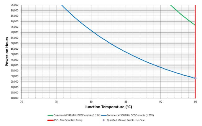
Figure 1. i.MXRT1020 commercial lifetime estimates, DCDC-enabled mode
