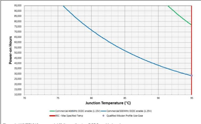
Figure 1. i.MXRT1010 commercial lifetime estimates, DCDC-enabled mode
