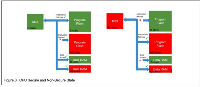
Secure and non-secure code runs on a single CPU for efficient embedded implementation.
