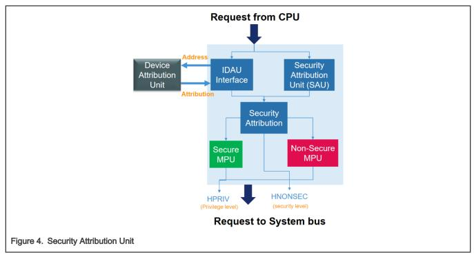
NXP incorporated an Implementation-specific Device Attribution Unit (IDAU) allowing a secure OS to be decoupled from the application.
