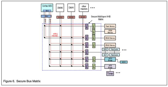
The Bus matrix between bus masters like the M33 core or DMA engines are wrapped with the MSW and have security side band signals used for tamper detection. There is a PPC for each bus slave port. The MPCs are used for memories and bus bridges.
