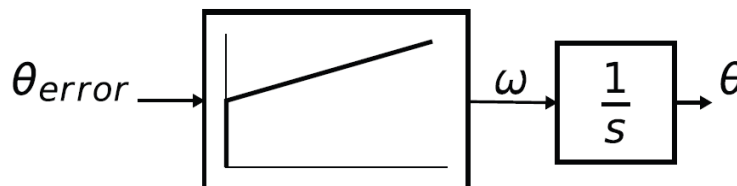
Figure 40. Block diagram of proposed PLL scheme for position estimation
