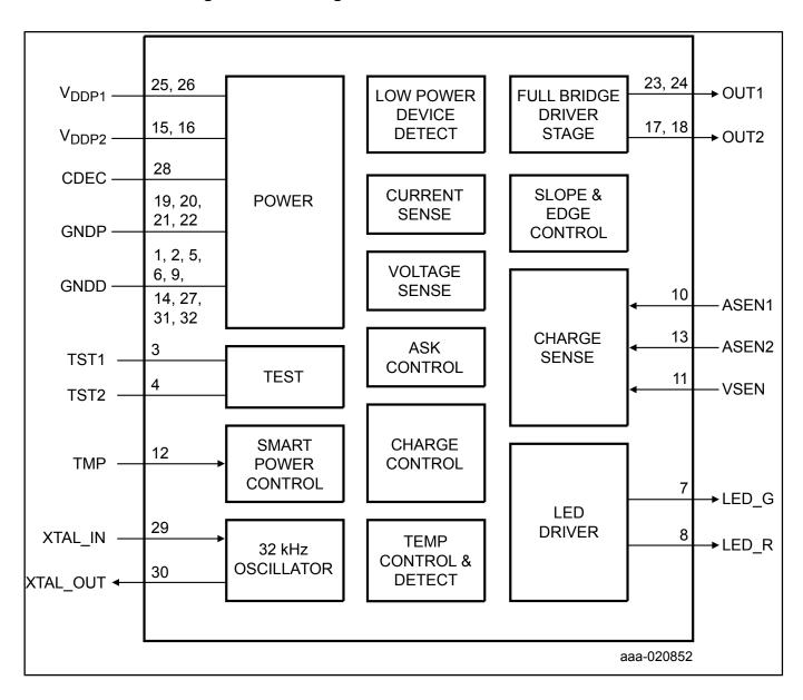
View additional information for Low-Cost One-Chip 5 V Qi Wireless Transmitter.
