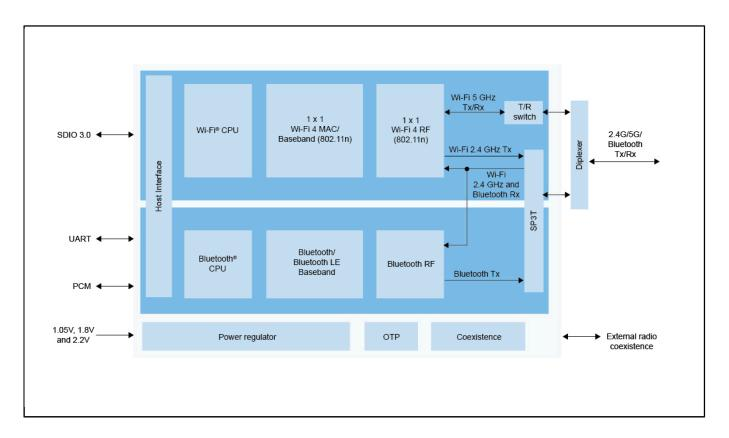
View additional information for 2.4/5 GHz Dual-Band 1x1 Wi-Fi® 4 (802.11n) + Bluetooth® 5.2 Solution.
