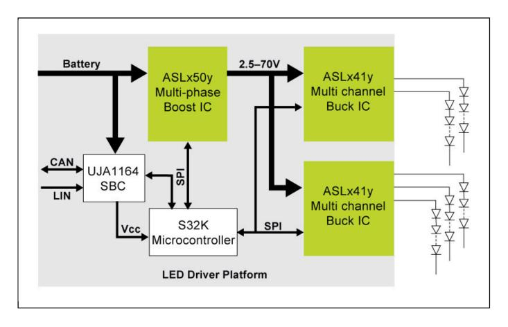
Single-Phase Automotive LED Boost Driver Block Diagram
