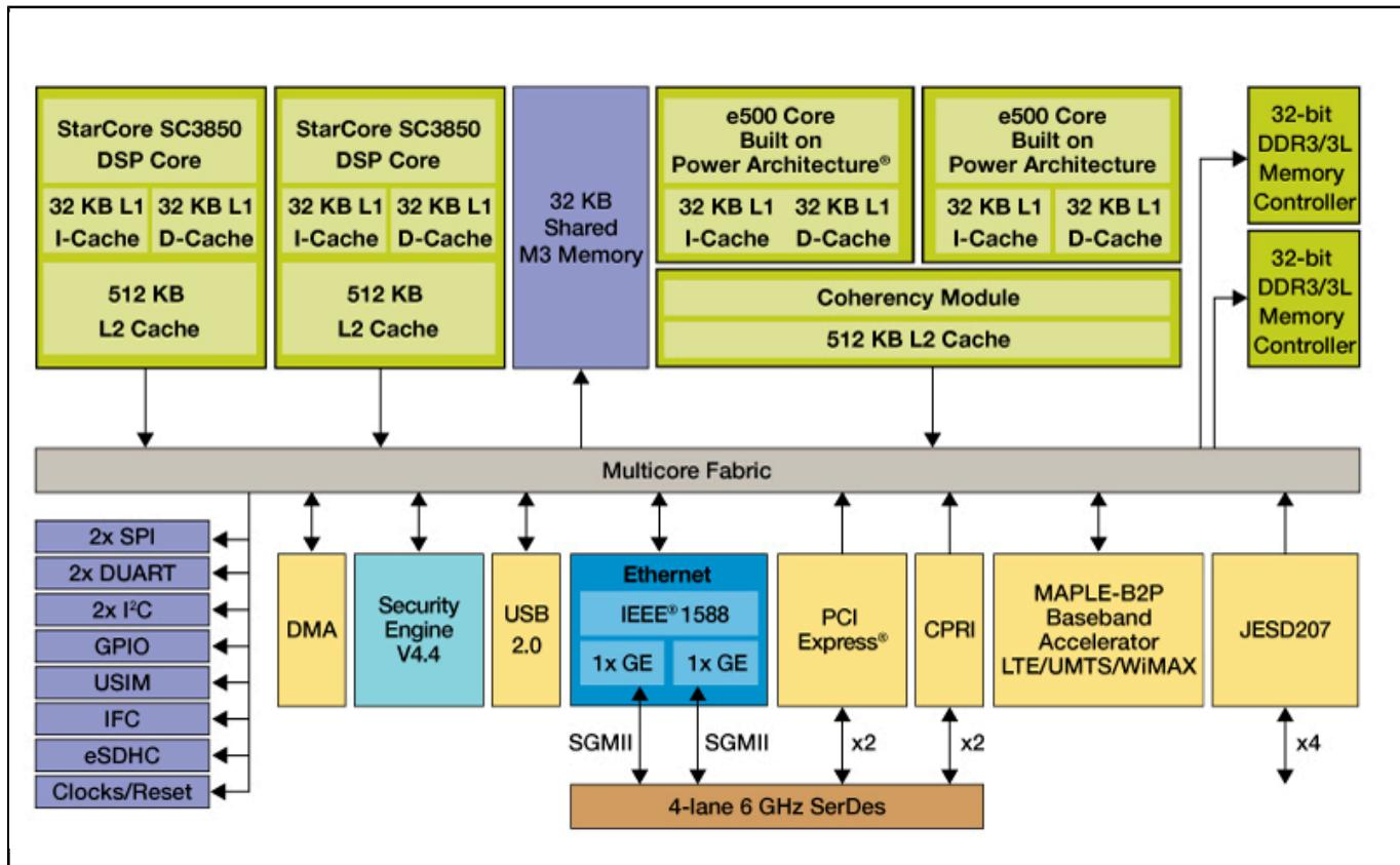
View additional information for [QorIQ® Qonverge BSC9132 Dual-Core Processor and Dual-Core DSP](#).
