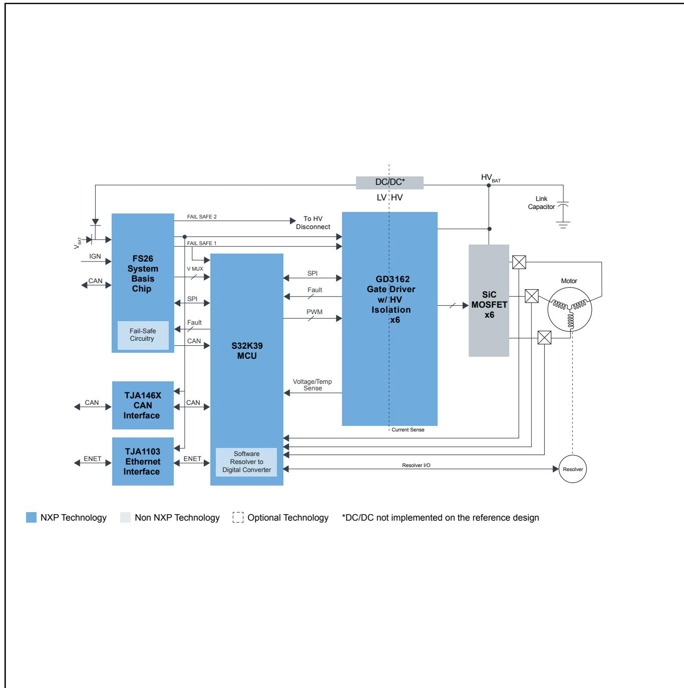
View additional information for [EV Traction Inverter Control Reference Design Gen 3](#).
