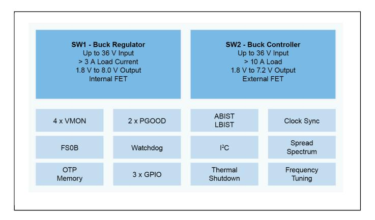
View additional information for Automotive Dual Buck Regulator and Controller with Voltage Monitors and Watchdog Timer.
