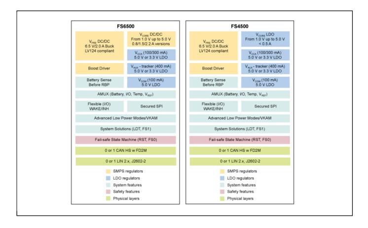
View additional information for Grade 1 and Grade 0 Safety Power System Basis Chip with CAN Flexible Data Transceiver.
