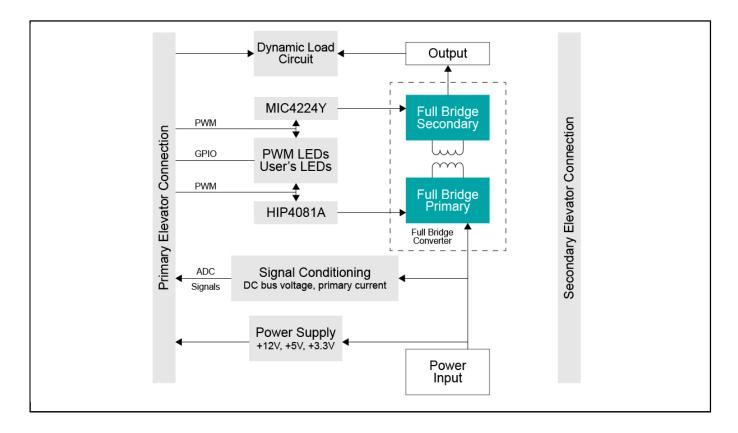
View additional information for KV Series Full-Bridge DC-DC Switch Mode Power Supply (SMPS).
