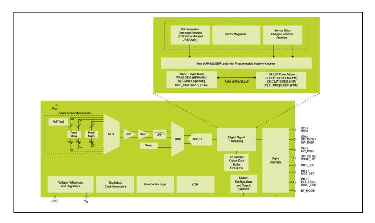
View additional information for ±2g/±4g/±8g/±16g, Low-Power 12-Bit Digital IoT Accelerometer.
