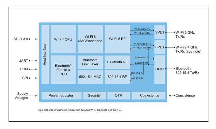
View additional information for 2.4/5 GHz Dual-Band 1x1 Wi-Fi® 6 (802.11ax) + Bluetooth® 5.4 + 802.15.4 Tri-Radio Solution.
