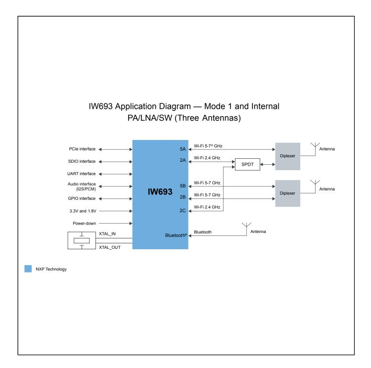
View additional information for 2x2 Dual-Band (5-7 GHz), 1x1 (2.4 GHz) Concurrent Dual Wi-Fi 6/6E and Bluetooth Combo Solution.
