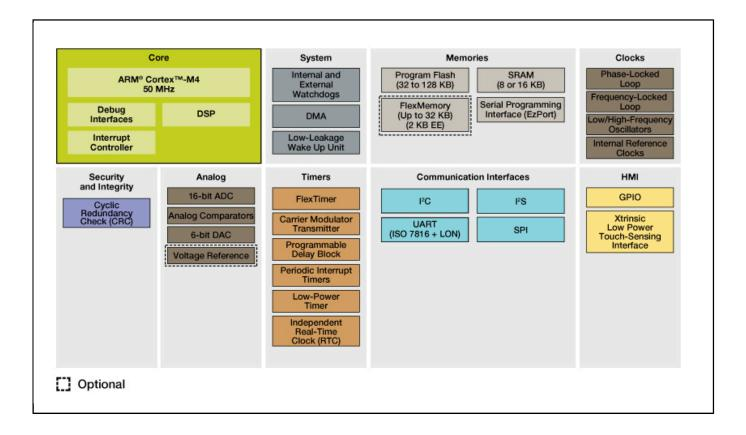
View additional information for Kinetis K10-50 MHz, Mixed-Signal Integration Microcontrollers (MCUs) based on Arm® Cortex®-M4 Core.
