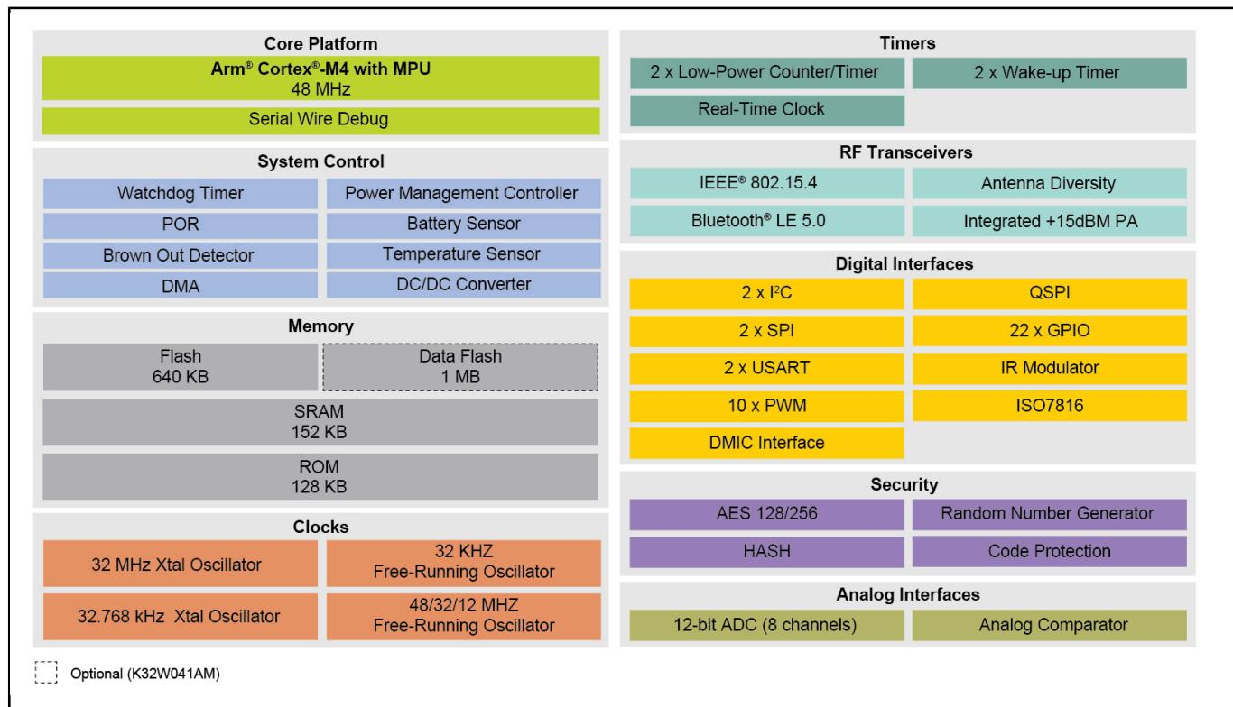
View additional information for [K32W041AM/A: High Performance, Secure and Low-Power MCU for Zigbee®, Thread™ and Bluetooth® LE 5.0 with High Tx Power Option](#).
