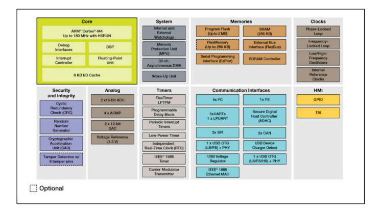
View additional information for Kinetis® K66-180 MHz, Dual High-Speed and Full-speed USBs, 2MB Flash Microcontrollers (MCUs) based on Arm® Cortex®-M4 Core.
