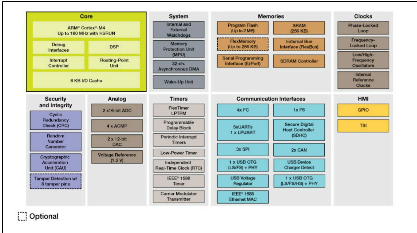
View additional information for [Kinetis® K66-180 MHz, Dual High-Speed and Full-speed USBs, 2MB Flash Microcontrollers \(MCUs\) based on Arm® Cortex®-M4 Core.](#)
