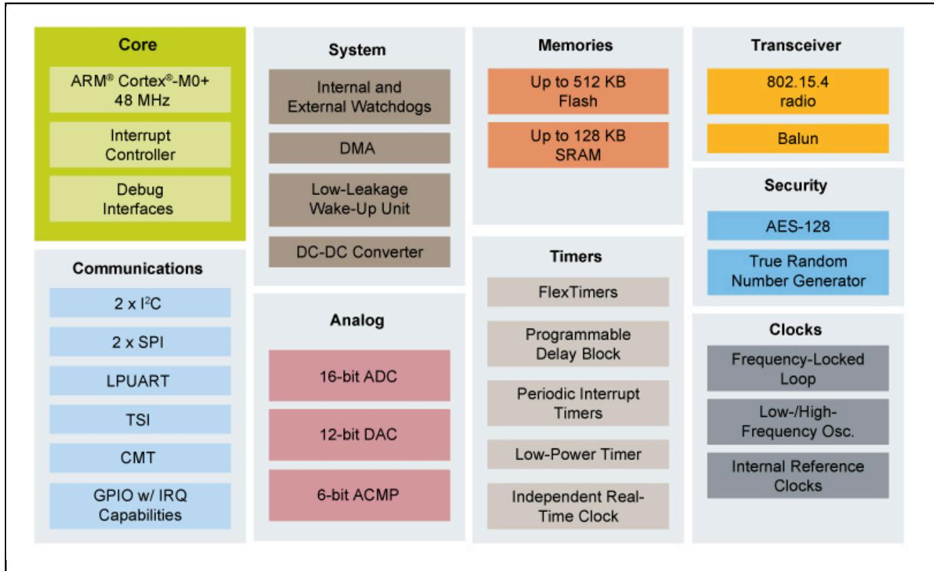
View additional information for [Kinetis® KW21Z-2.4 GHz 802.15.4 Wireless Radio Microcontroller \(MCU\) based on Arm® Cortex®-M0+ Core.](#)
