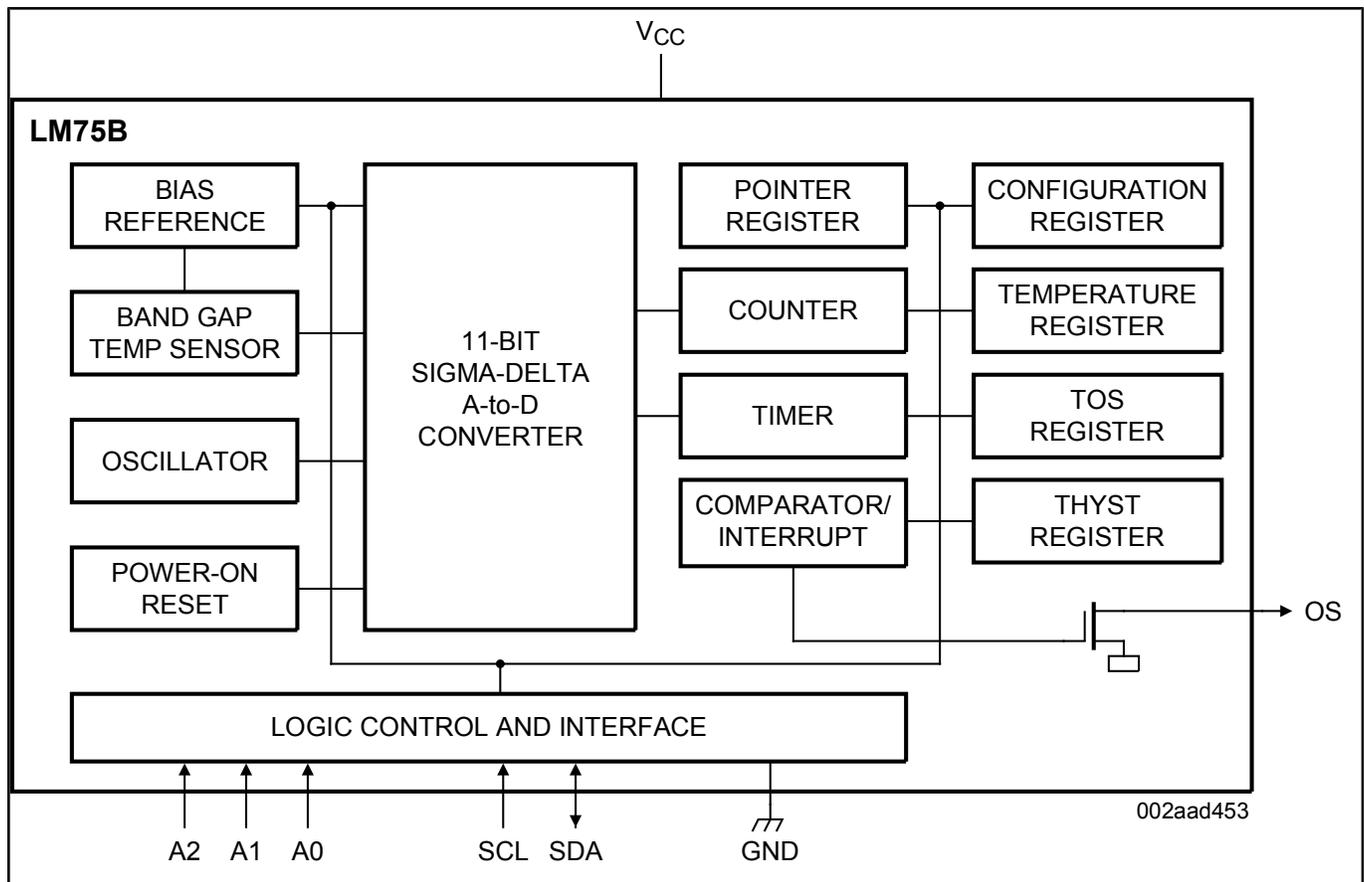
View additional information for [Digital Temperature Sensor and Thermal Watchdog](#).
