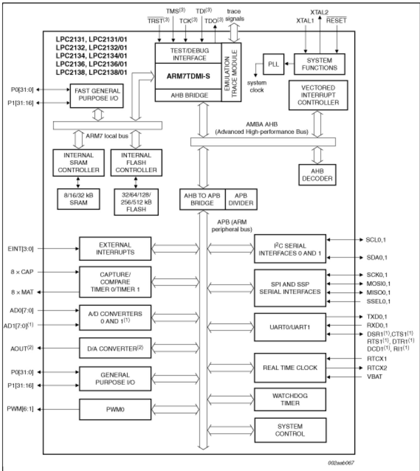
View additional information for [Single-chip 16/32-bit microcontrollers; 32/64/128/256/512 kB ISP/IAP flash with 10-bit ADC and DAC.](#)
