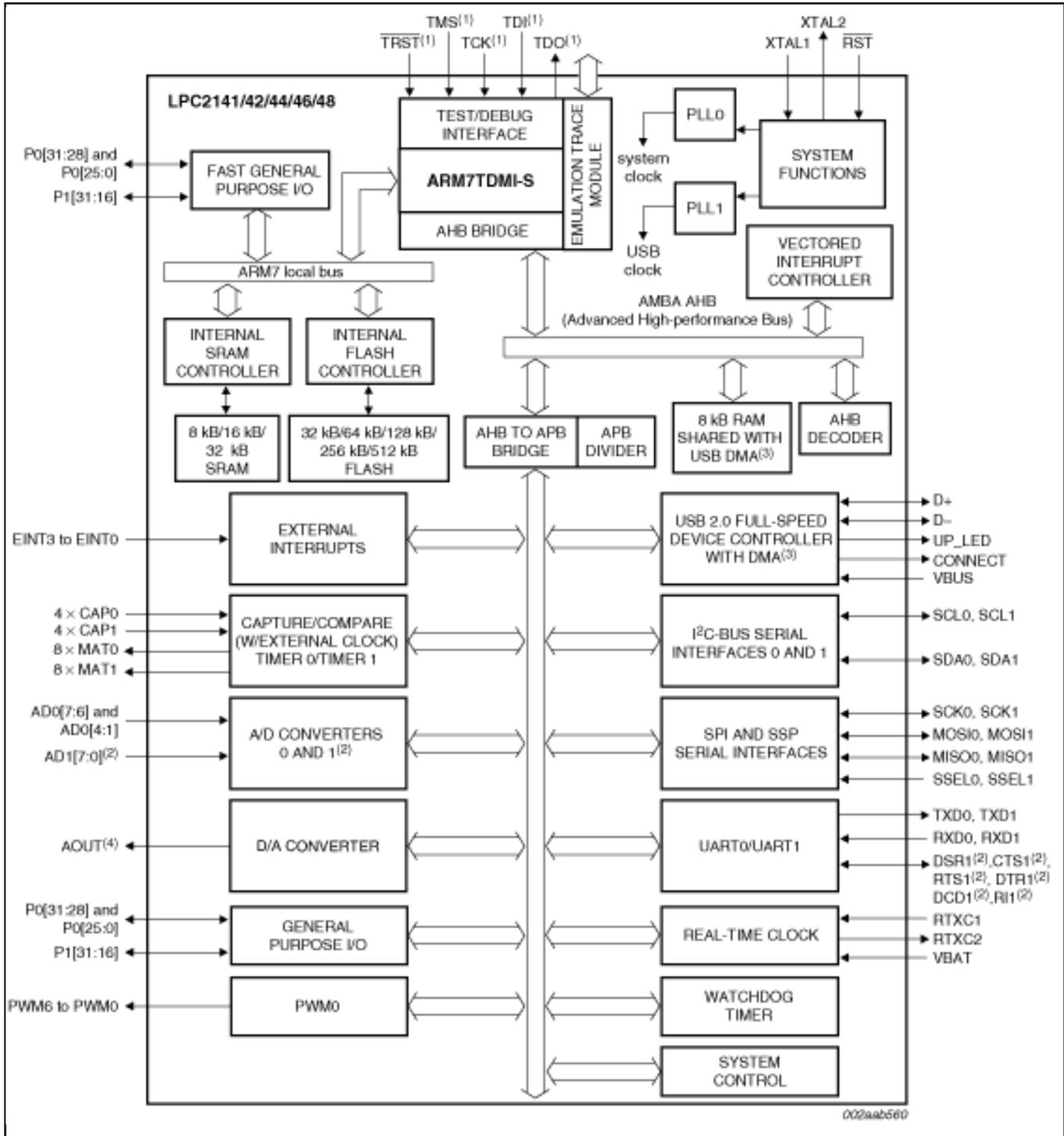
View additional information for [Single-chip 16-bit/32-bit microcontrollers](#); up to 512 kB flash with ISP/IAP, USB 2.0 full-speed device, 10-bit ADC and DAC.
