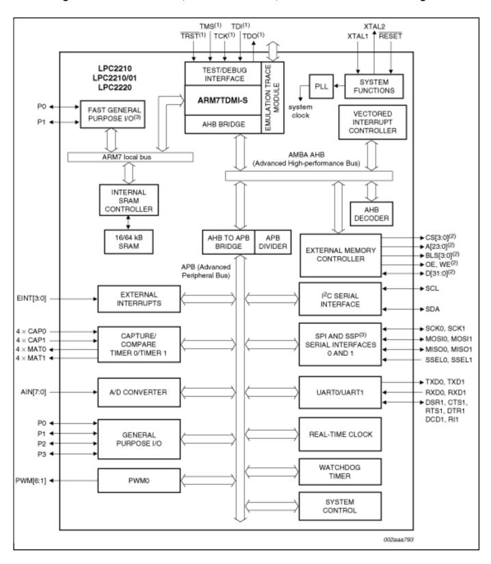
View additional information for 16/32-bit Arm® microcontrollers; flashless, with 10-bit ADC and external memory interface.
