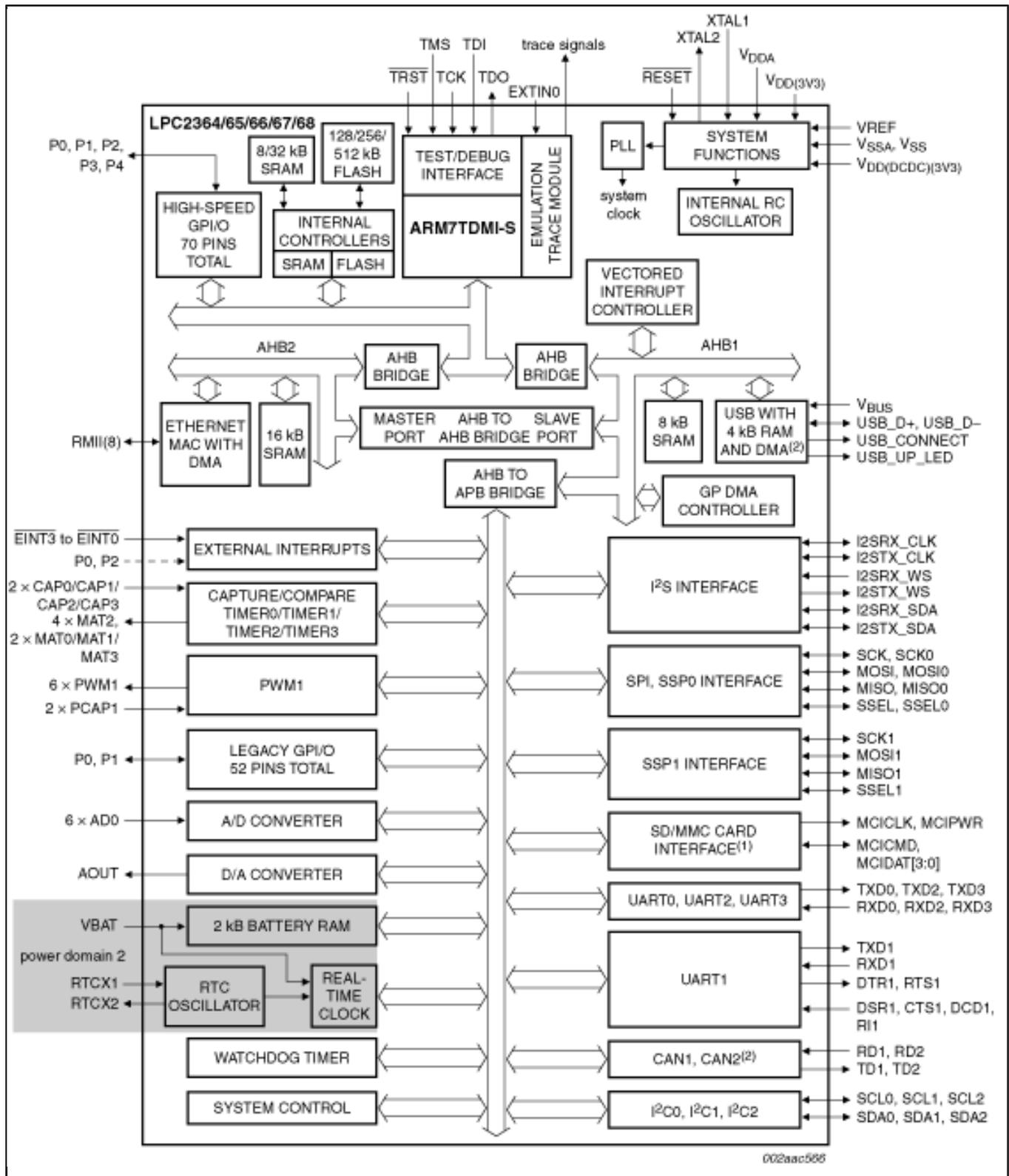
View additional information for [Arm7™](#) with 256 kB flash, 58 kB SRAM, Ethernet and 10-bit ADC.
