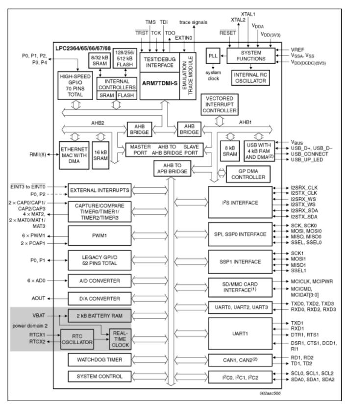
View additional information for Arm7<sup>™</sup> with 512 KB Flash, 58 KB SRAM, Ethernet, USB 2.0 Device, CAN, SD/MMC, and 10-Bit ADC.
