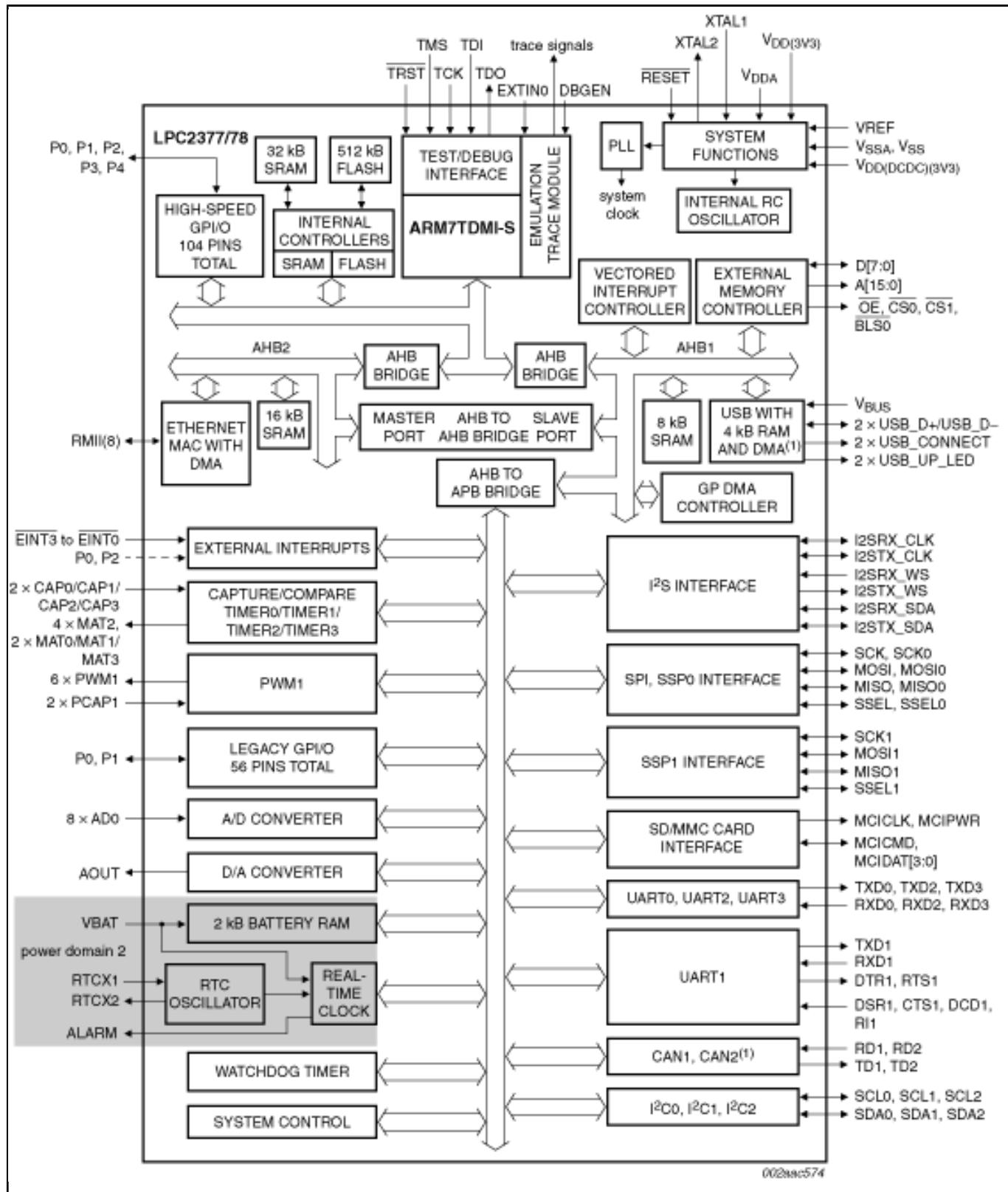
View additional information for **Arm7™** with 512KB flash, 58 KB SRAM, Ethernet, and 10-bit ADC.
