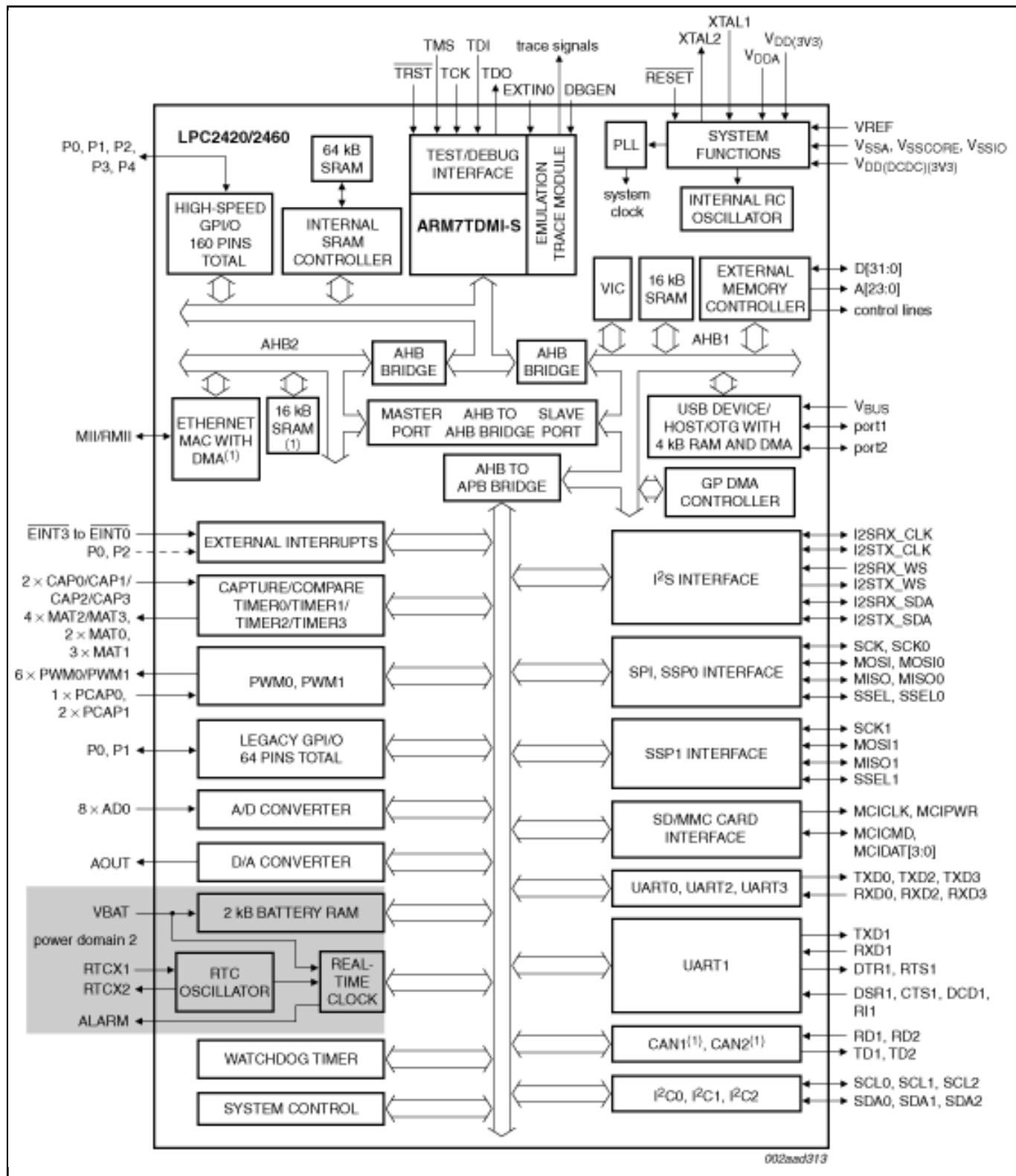
[View additional information for Flashless 16-bit/32-bit microcontroller; Ethernet, CAN, ISP/IAP, USB 2.0 device/host/OTG, external memory interface.](#)
