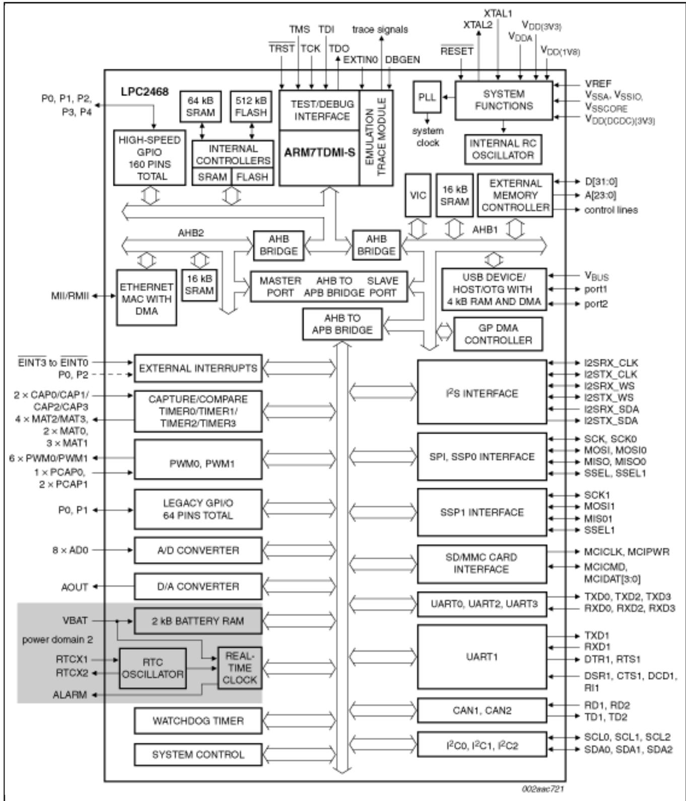
View additional information for [Single-chip 16-bit/32-bit micro; 512 kB flash, Ethernet, CAN, ISP/IAP, USB 2.0 device/host/OTG, external memory interface](#).
