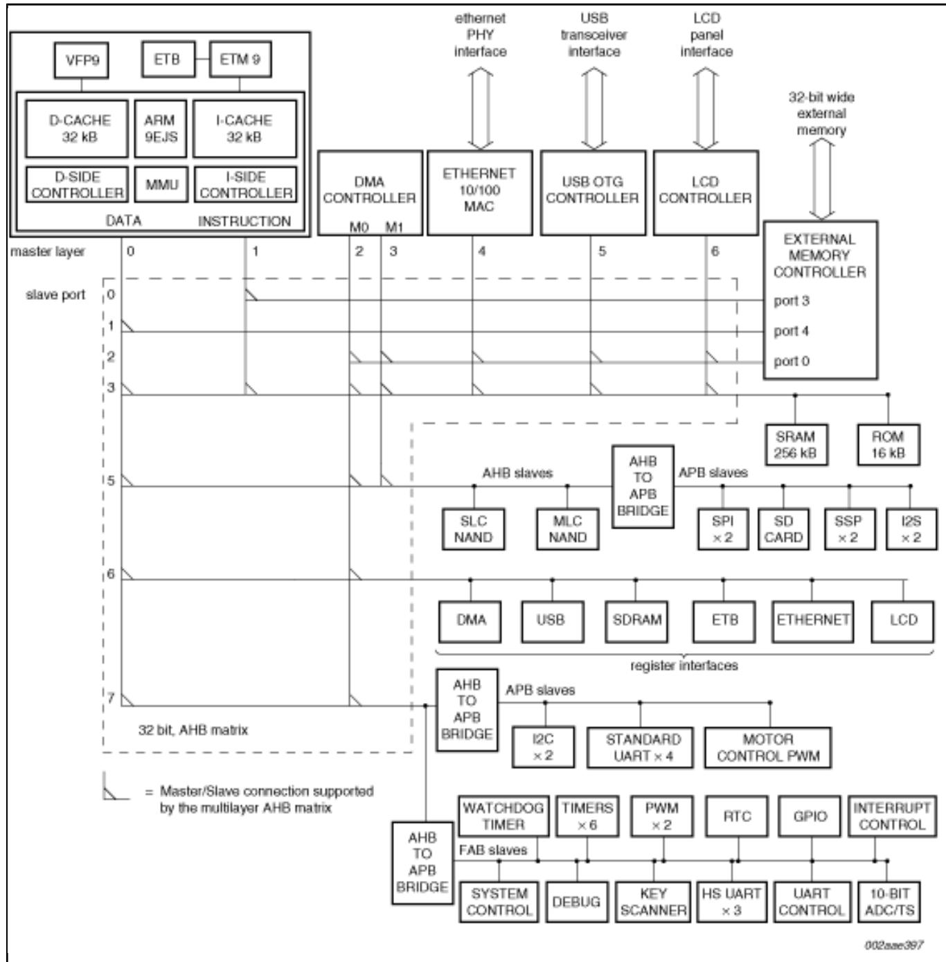
View additional information for [Arm926EJ-S™ with 256 KB SRAM, USB High-Speed OTG, SD/MMC, Nand Flash Controller, Ethernet, LCD Controller](#).
