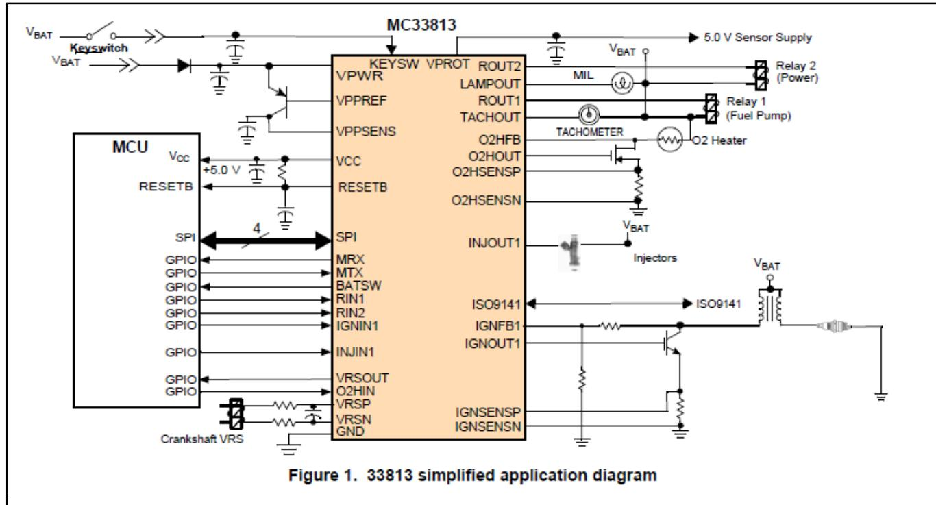
[View additional information for One Cylinder Small Engine Control IC.](#)
