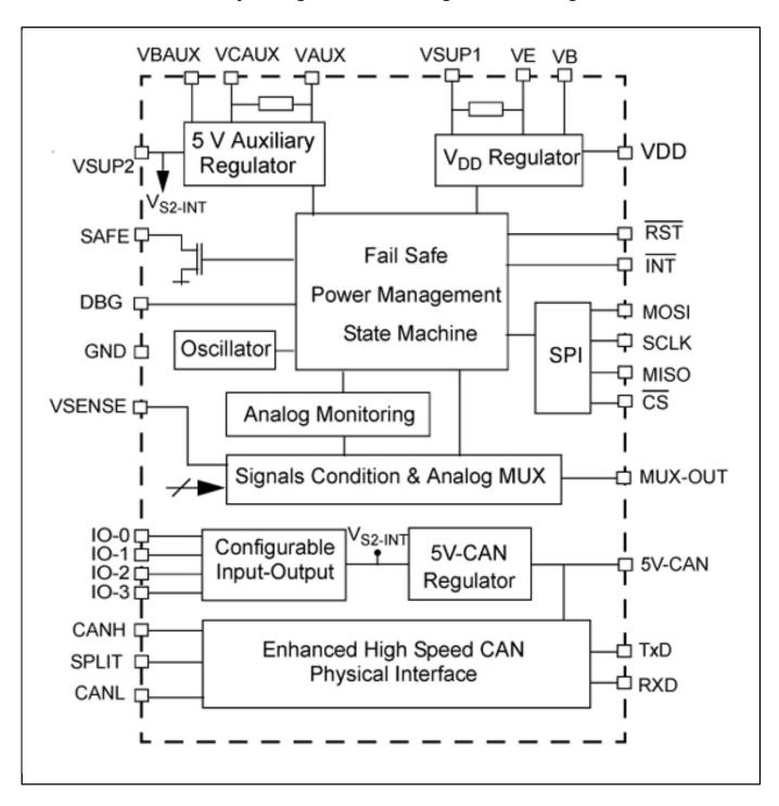
View additional information for System Basis Chip Gen2 with High Speed CAN.
