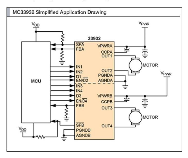
View additional information for H-Bridge Motor Driver, 5-28 V, 5 A, 11 kHz.
