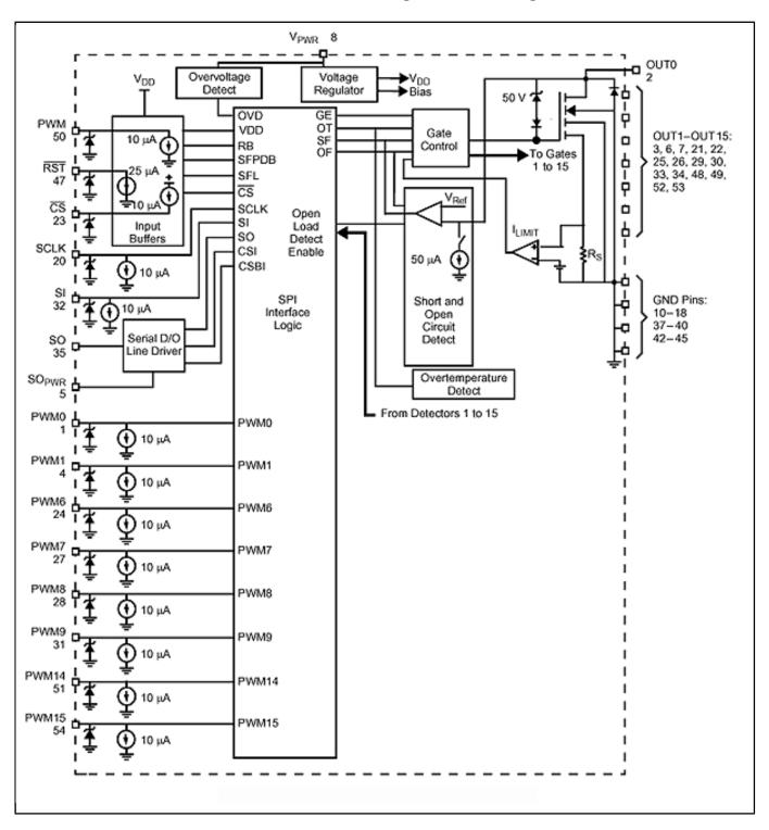
View additional information for 16-Output Switch with SPI and PWM Control.
