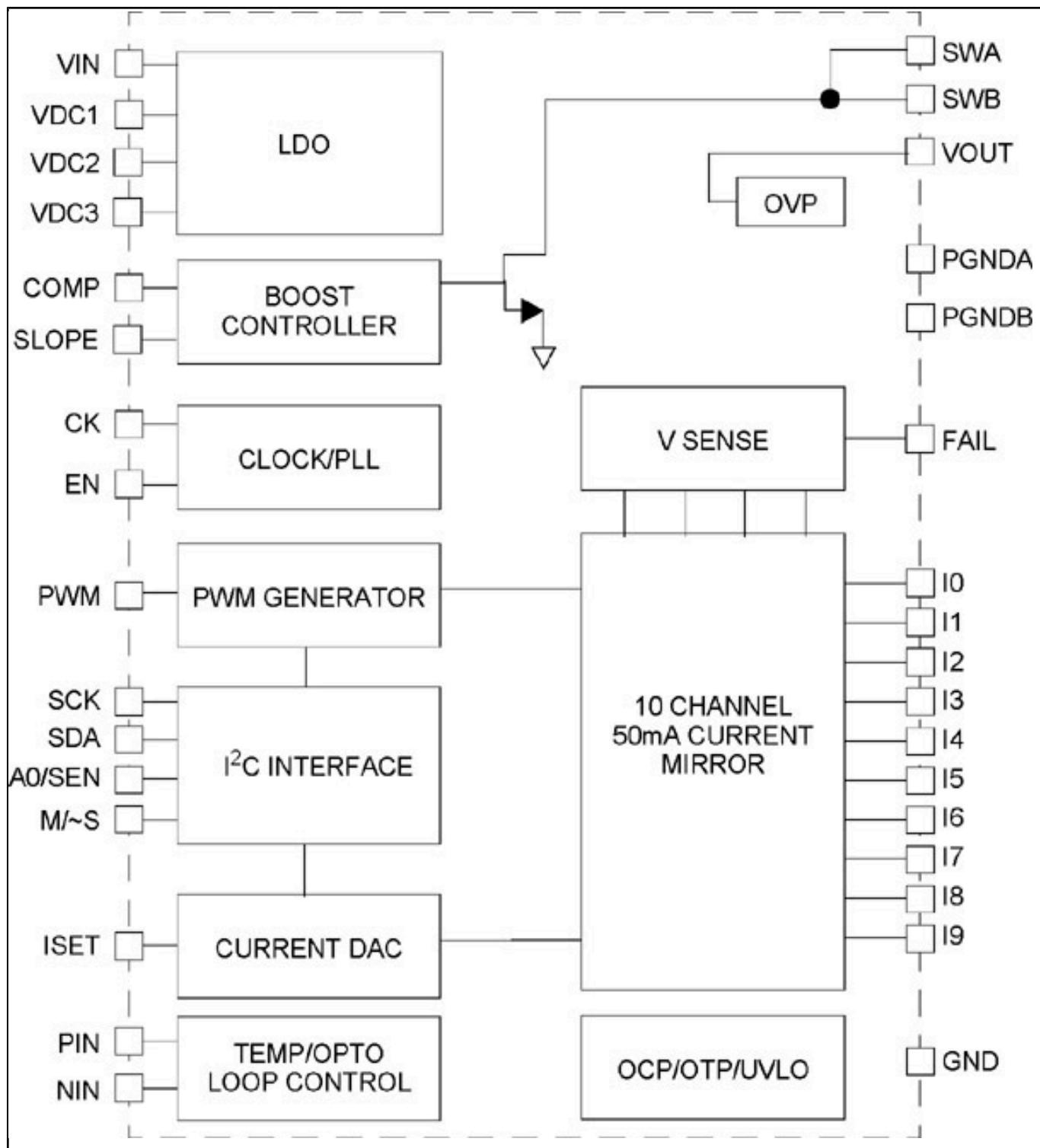
View additional information for [10 Channel LED Backlight Driver with Power Supply](#).
